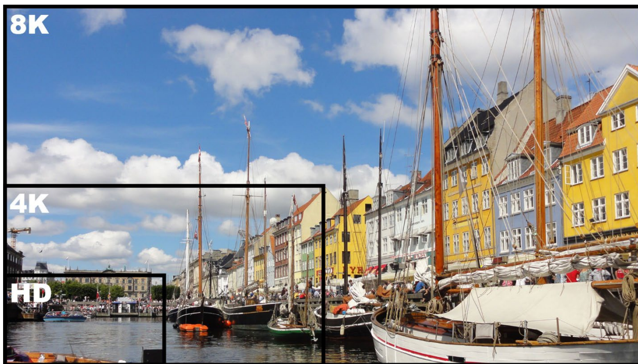
8K delivers four times the pixels of 4K and sixteen times the pixels of Full HD.
